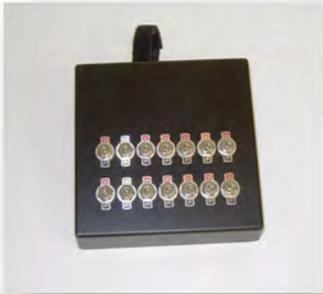
Mechanical cut-off switches may be provided as an alternative to phone shut down using the system workstation. These manual overrides or “kill switches” are used to quickly turn the telephones on/off on demand. Multi-phone kill switches will be installed at each control center or as specified by the facility.
