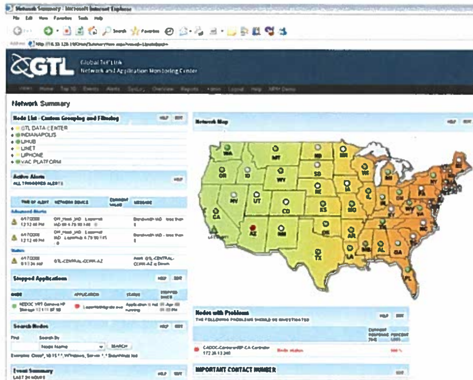
SNMP interface displays current network status and access to historical statistical data.
